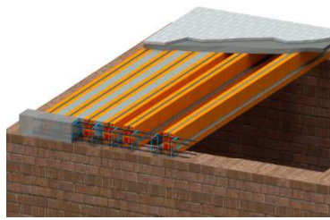
Fig. 15. Floor with prefabricated reinforced hollow clay tile beams with RC ring beams
