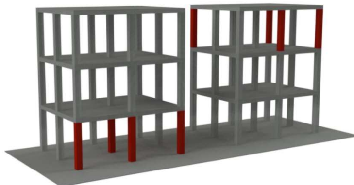
Fig. 55. Example of RC frames with same quantity of damaged structural elements but different residual seismic capacity
