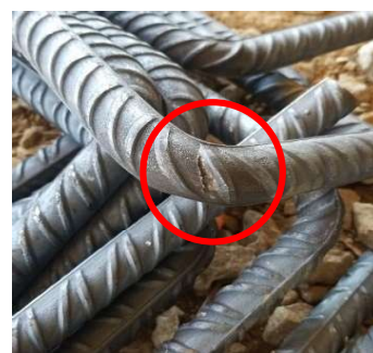
Fig. 32. Cracks in steel rebars
